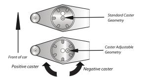
Figure 1: Outer Bush Caster Adjustment
