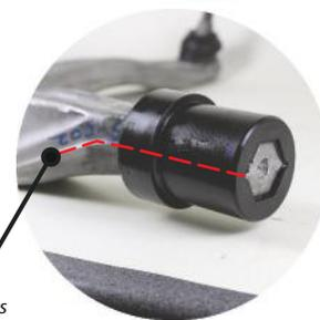
Align the slots with the casting line on arm
