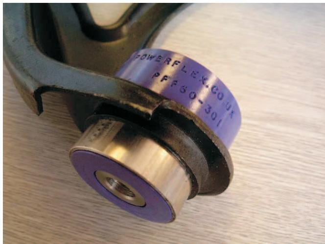
Fig 2: Bush fitted in wishbone
