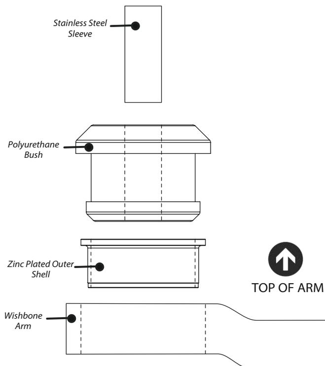
Figure 1 - diagram showing how the parts will fit together inside the arm
