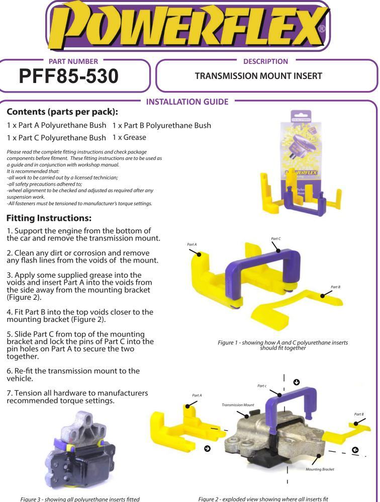
Figure 3 - showing all polyurethane inserts fitted inside the transmission mount
