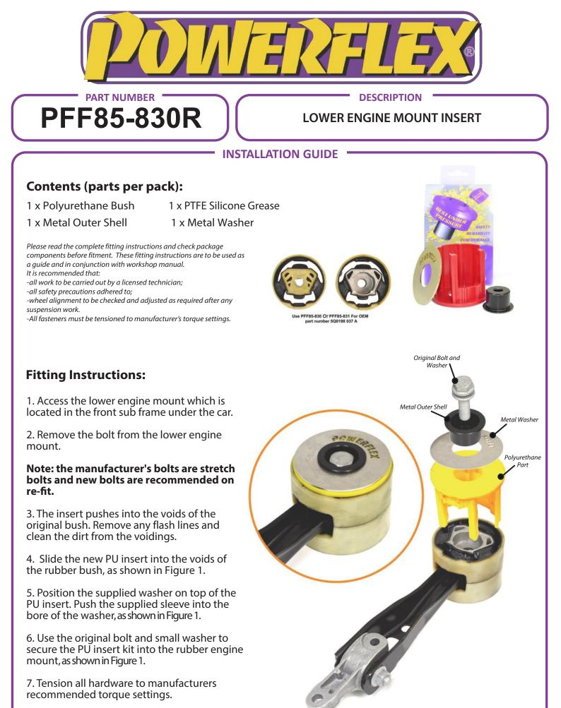
Figure 1 - assembly of PFF85-830 in the engine mount
