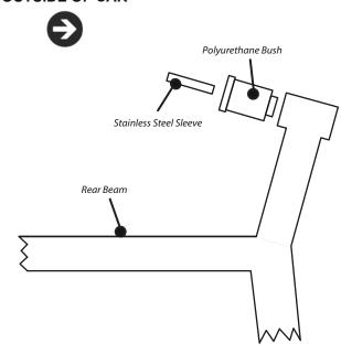
Figure 1 - how the polyurethane bush fits in the rear beam (top view)
