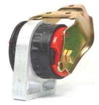
Figure 4 - showing polyurethane insert fitted inside the engine mount
