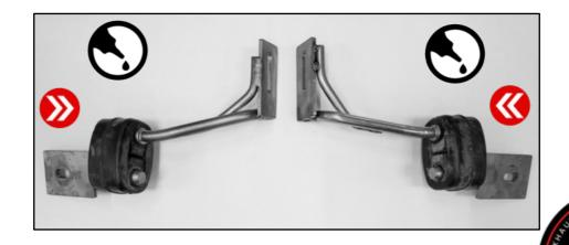
Dismount the actuators from the stock rear exhaust and mount them onto the REMUS valve tubes.
