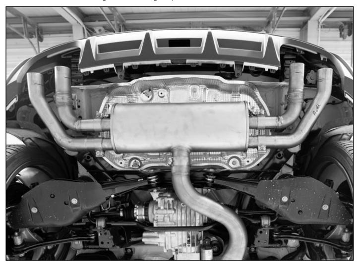
Align the REMUS front silencer and tighten all connections.
