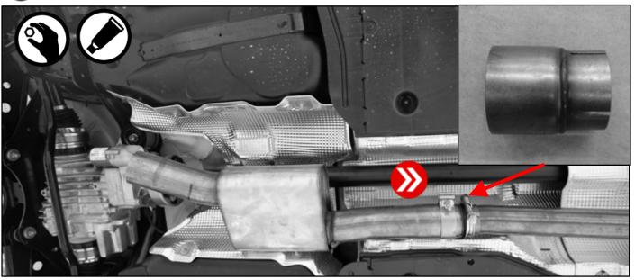
Mount the bracket onto the rubber hanger.
