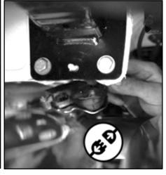
Unhook the rubber hanger, dismount the cross strut and remove the stock rear exhaust.
