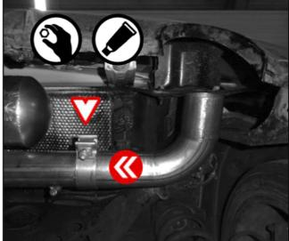
Slip On and mount the REMUS Tail pipes onto the outlet.
