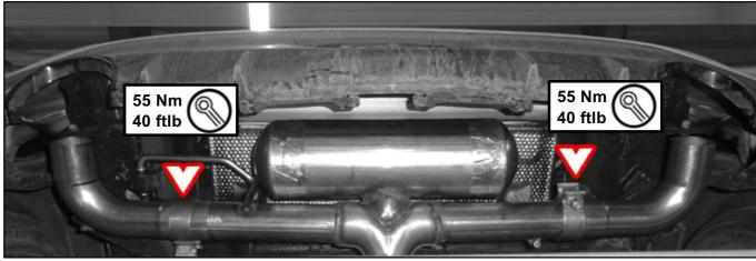
Slip On and mount the REMUS Tail pipes onto the outlet.
