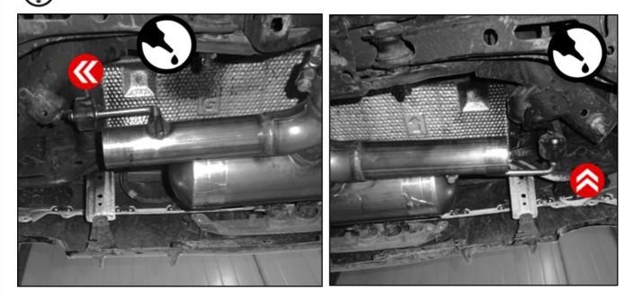
Install the two outlet tubes onto the REMUS sport exhaust.
