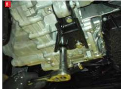
Remove rear propshaft bolts and mark the position of rotation.
