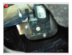
33) If you have the Scorpion cat back system, you will need to fit the original valve onto the valve plate as shown here.
