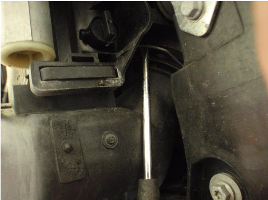
11. On the drivers side of the intercooler, depress the clip holding the intercooler to the car with a flat bladed screwdriver. At the same time, push the intercooler to the left (looking from the front of the car) to release it from the bracket on the passenger side, then pull down to release the passenger side connector.
