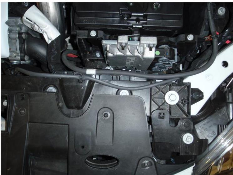
4. Undo the six T20 screws on the top of the bumper.
