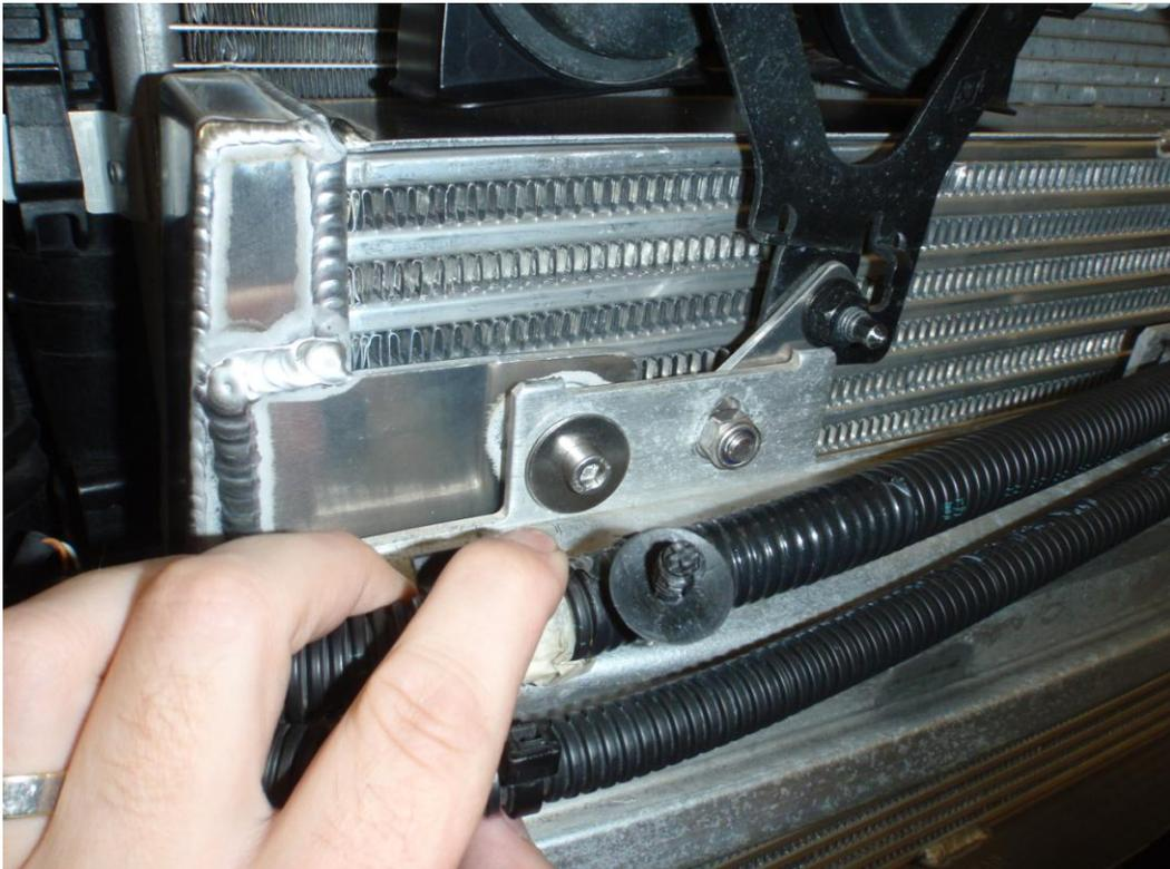
18. Your intercooler should now be fitted and bolted in firmly. The top ducting (step 8) now has nothing to clip to and hold it in place when you reassemble the bumper. We used a very small piece of sticky tape to hold it in place to the condenser whilst the bumper was fitted on top of it. Refit the bumper following steps 8-1 in reverse order. No trimming is necessary. Enjoy your new found performance !
