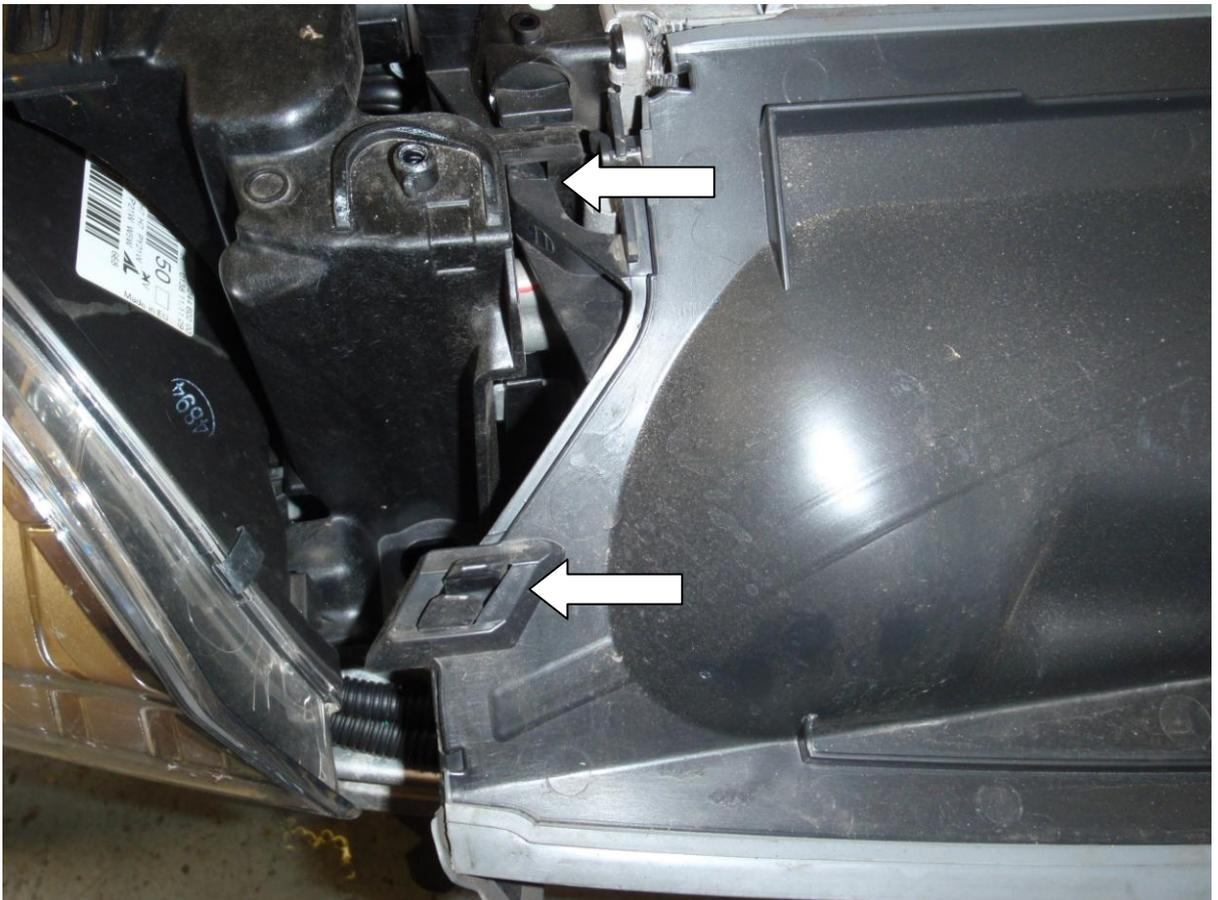
9. Unclip the electrical connection to the horn by squeezing the metal retainer, and remove the single 10mm nut holding it to the crash bar.
