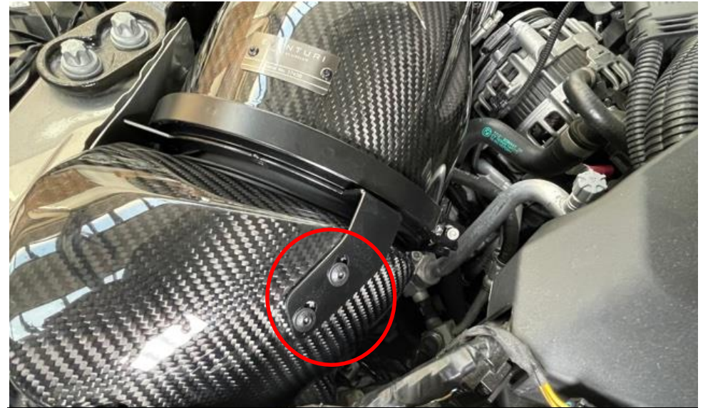
41. Using the supplied M5 screws - secure the bracket to the duct.
