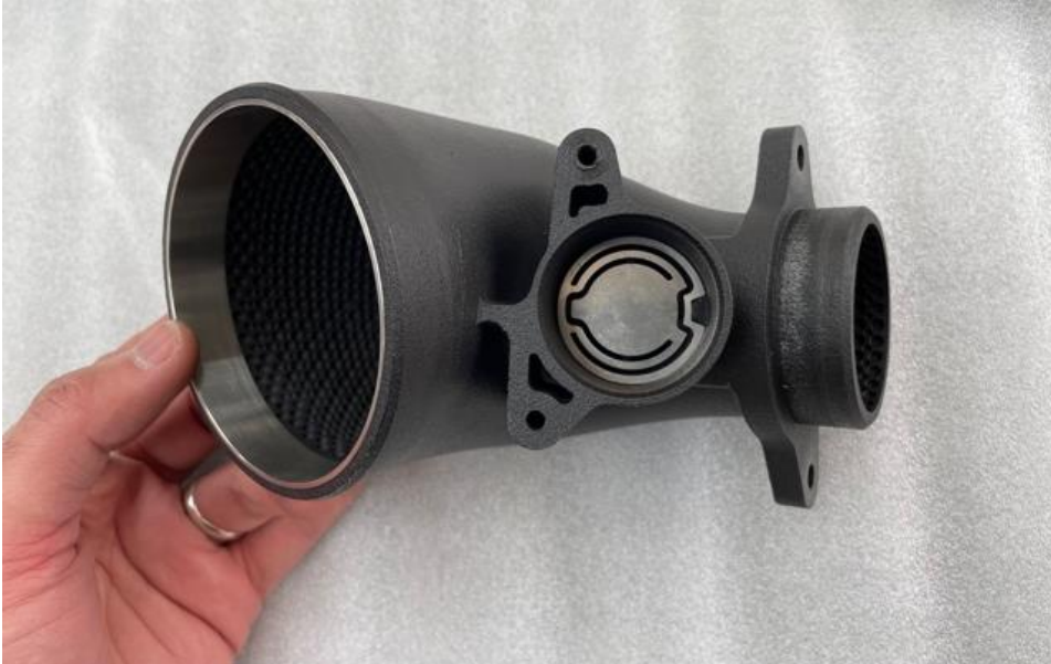
13. Insert the metal shim into the new inlet as shown. The notch should line up with the tab on the inside.
