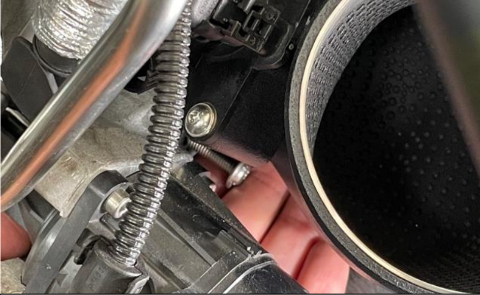
20. Position the screw into the hole and then using an appropriate extension, start to turn it carefully to catch the threads.
