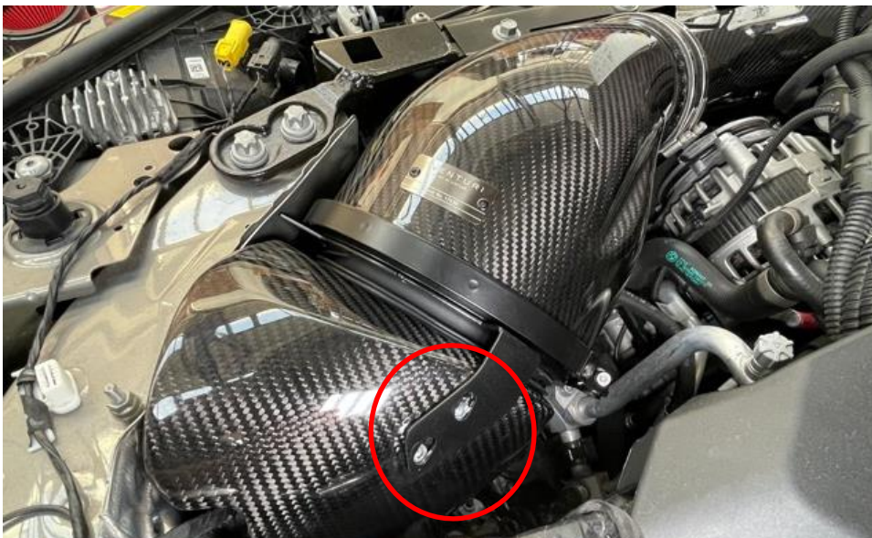
38. Rotate the housing so that the holes in the bracket line up with the inserts on the duct.
