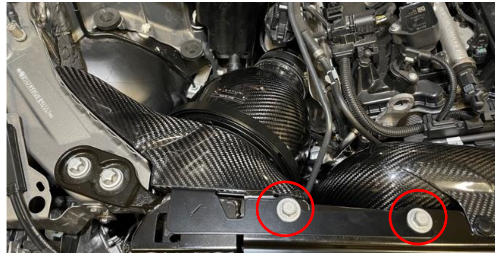
59. Insert the 2 x stock bolts previously removed and tighten.
