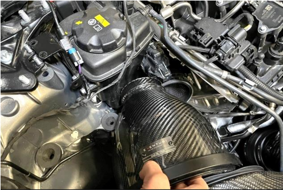
56. Lower the housing down past the turbo actuator and at the same time lower the coolant tank.
