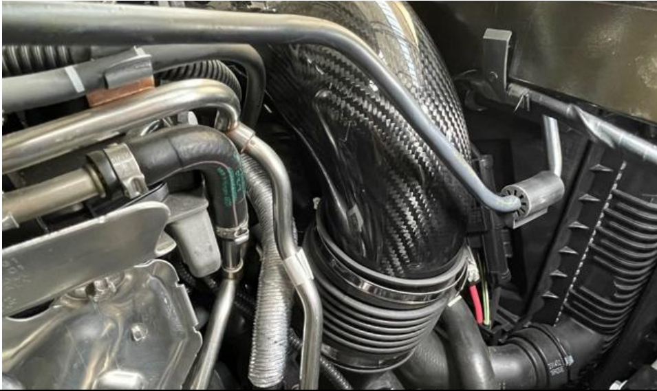
36. Push the carbon tube into the flexible hose ensuring it goes in all the way around.
