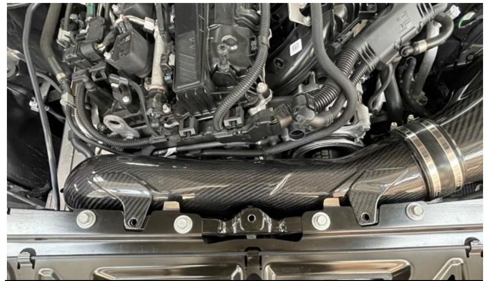
37. Remove the cloth and rotate the tube so that the carbon brackets sit flat on the slam panel.
