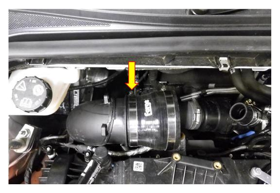
12. Fit the Forge alloy intake to the silicone reducer and silicone diverter valve hose. Use the hose clamps to secure it. Re attach the oil breather pipe and tighten the cam cover fastener to the mounting bracket on the intake pipe.
