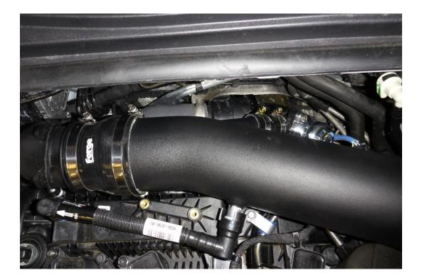
. Re fit the MAF to the MAF boss on the intake pipe.
