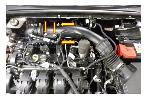
3. Using a 7mm ratchet and socket remove both hose clamps at each end of the intake pipe. You will now be able to pull the intake pipe out of the engine bay.
