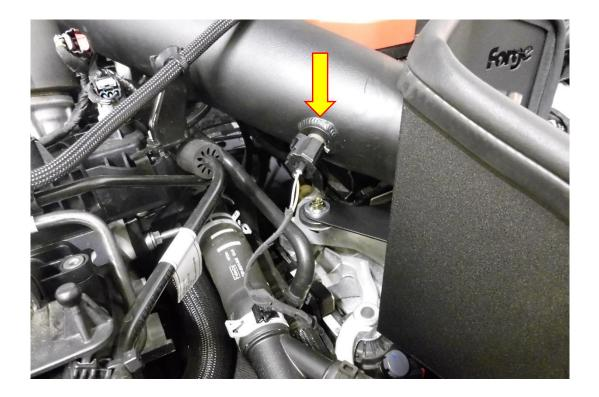
**14**. Fit the air filter to the intake pipe and using a 7mm socket and ratchet secure the filter in place.
