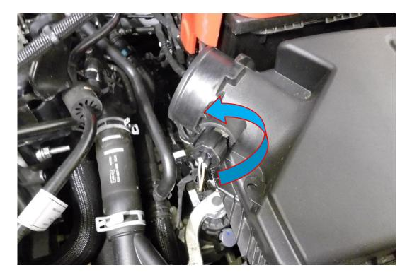
5. Remove the X2 plastic fasteners attaching the air scoop to the slam panel. The air scoop will now pull away and the airbox can be removed at the same time by pulling sharply upwards allowing both items to be removed in situ.
