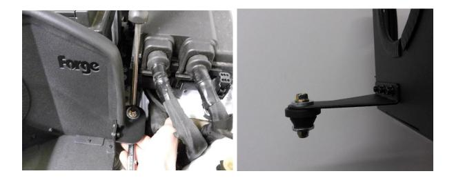
9. Using an 8mm spanner loosen off the cam cover fastener in the picture below.
