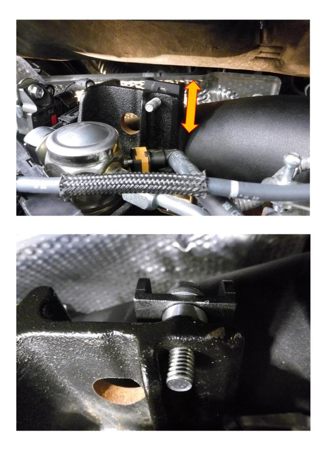
12. Re-install the vac line to the brass 4mm hose joiner on hose #2046 use the supplied cable tie to secure it in place. Using a 7mm socket and ratchet and hose clamp 16-27 attach the oil breather pipe to the barbed spout from hose #2046.
