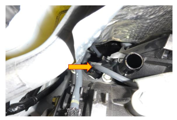
8. Using a 12mm socket and rachet or 12mm spanner remove the M8 fastener and M8 nut attaching the turbo elbow to the turbo. Using an E8 socket and rachet remove the threaded M8 stud from the turbo. Loosen the hose clamp at the other end of the turbo elbow, the turbo elbow can now be parted from the hard pipe and can be removed from situ.
