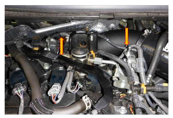
**15**. Please fully check your installation and ensure all fasteners are tight with no mis fit as a loose hose can activate the engines EML (Engine management light). Fit the engine cover to complete the installation of FMTIA8. Take your vehicle for a test and enjoy your new Forge Motorsport product.
