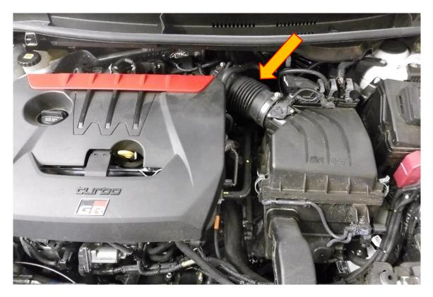
2. Using a 10mm socket and rachet loosen both hose clamps attaching the OEM turbo inlet hose. The oil breather hose can will simply pull off to remove from situ.
