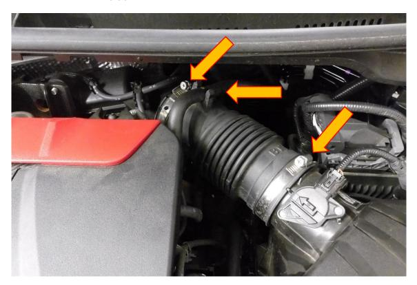
3. Detach the vacuum lines from the turbo inlet hard pipe clips shown by the arrowes below.
