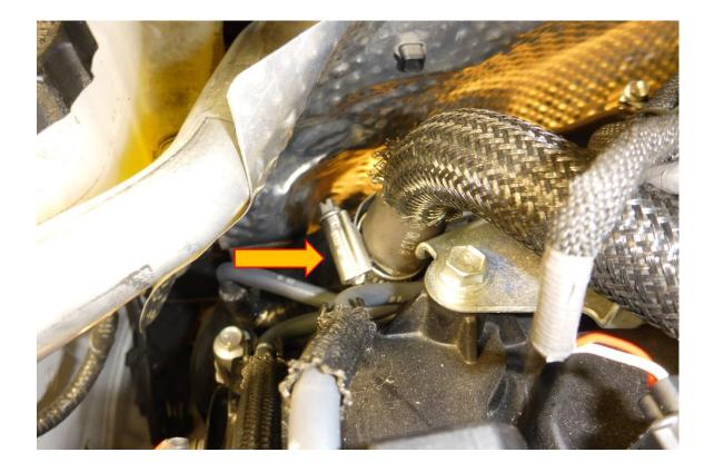
**13**. Using a 7mm socket and ratchet and the remaining hose clamps fit hose #2045 to the hard pipe and air box. Hose clamp 80-100 should be fitted at the hard pipe end and hose clamp 70-90 should be fitted airbox end.
