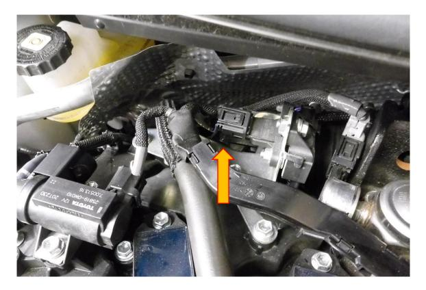
6. Using long nose plyers loosen the sprung hose clamp to allow you to remove the oil breather pipe.
