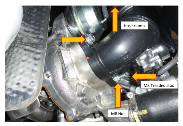
9. With the OE turbo adaptor removed pull the original red rubber O- ring out of its housing. Fit the O ring to the Machined coupler from the Forge kit. Using a 6mm Allen key and the supplied M8 cap head fasteners from the FMTIA8 kit, fit the Forge Motorsport machined billet adaptor to the turbo.
