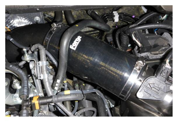
14. Re-route the vac hose which was originally attached to the OEM intake pipe. Use the supplied cable ties to secure it in place.
